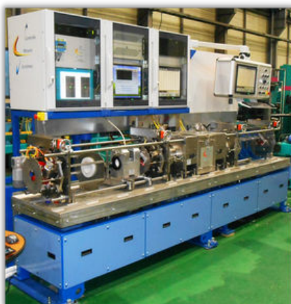
HIGH PRECISION TUBE ROTARY HEAD INSPECTION
