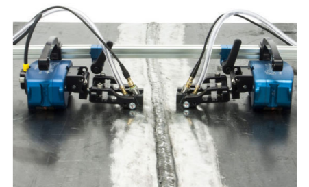
Phased Array Weld Inspection
