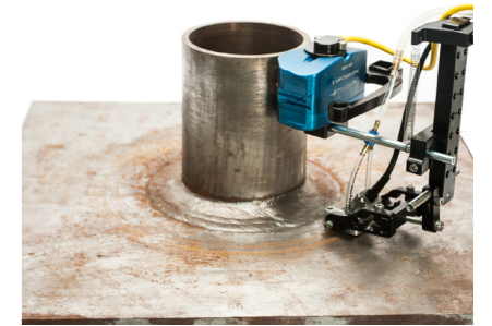
Phased Array Nozzle Inspection
